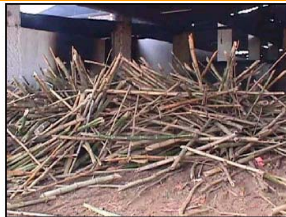
Bamboo used to fire bricks
