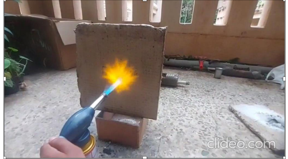
Biomass Panel treated by Sodium Silicate solution
