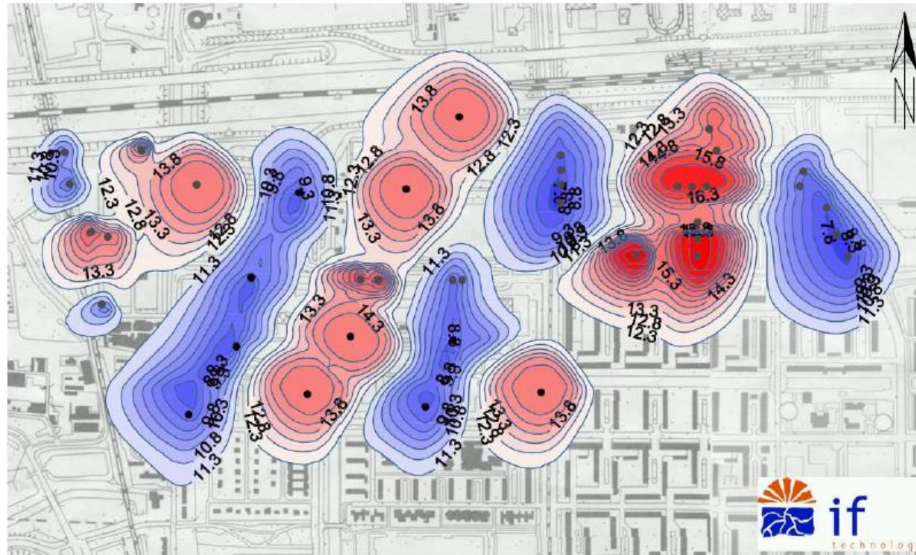
An example of placing the warm and cold wells parallel to the southwestern groundwater flow at the Zuidas in Amsterdam (IF Technology).
