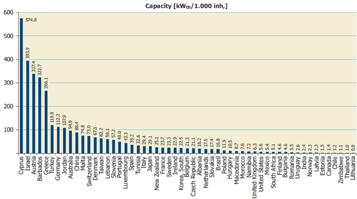
**Figure 7:** Total capacity of glazed flat plate and evacuated tube collectors in operation in kW<sub>th</sub>
