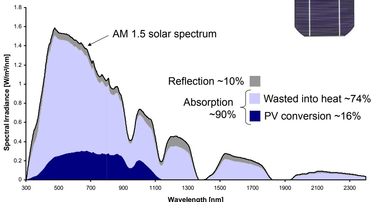
Graphical representation based on actual measurements (reflection, EQE and I-V)
